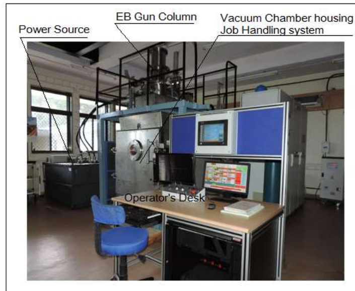
Figure 2: Photograph of 12kW, 80kV electron beam welding machine installed at BARC
