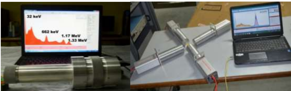
Fig. Pulse height spectrum of a single and four coupled portable gamma spectrometer radiation detectors using CsI:Tl crystal (MCA in these detectors are imported and can be replaced by indigenous ones)
