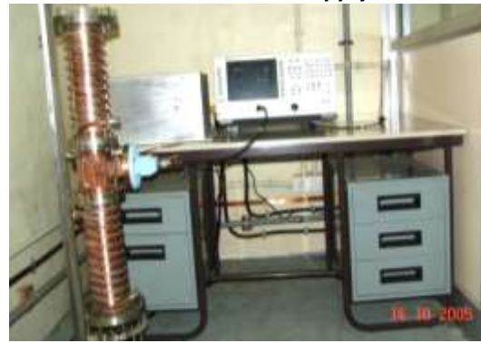
RF LINAC cavity under RF testing Design Values of 10 MeV Cavity Structure Frequency: 2856 \pm 2 MHz, VSRW = 2.0
