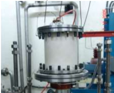
Electron Gun, 70 keV, 1 A, 10 \mu s, 400 Hz Cathode: LaB6, Configuration: Triode Emission: Thermionic
