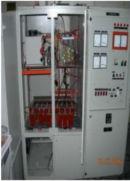
E-Gun Modulator (50 kV, 1 A, 400 Hz, 10 \mu s)
