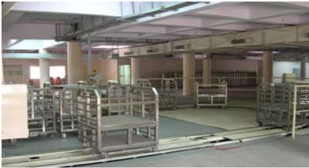
Conveyorsystem, Variablespeed: 1 – 7 m/min
