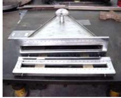
Scan magnet and Scan Horn, 200 X 279 x1000 mm (H), Ti Foil – 50 microns
