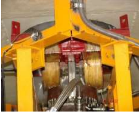
Scan magnet and Scan Horn, 200 X 279 x1000 mm (H), Ti Foil – 50 microns
