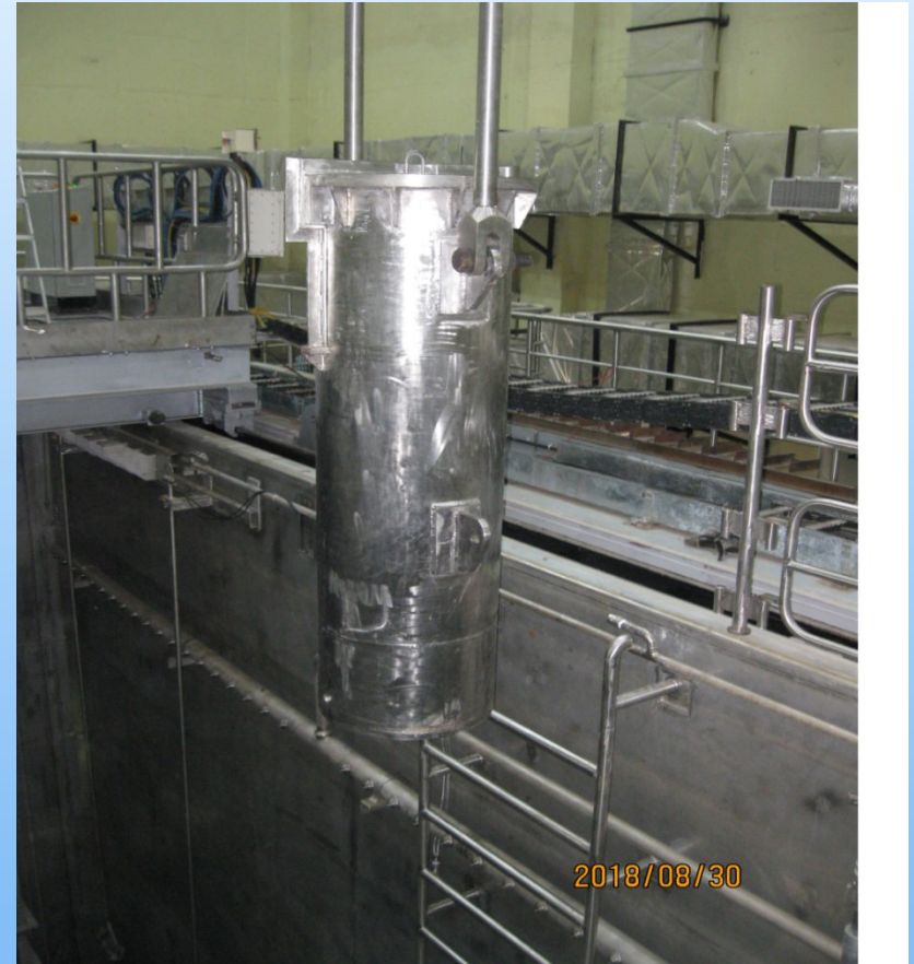
Handling trials of Isotope shielded flask in the Apsara pool .
