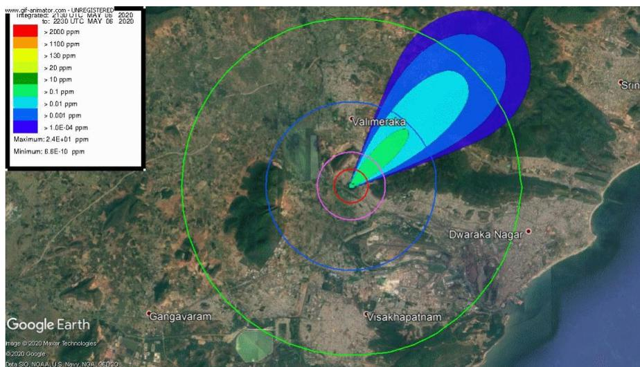
Figure-5: Styrene concentration (ppm) around LG Polymer Plant
