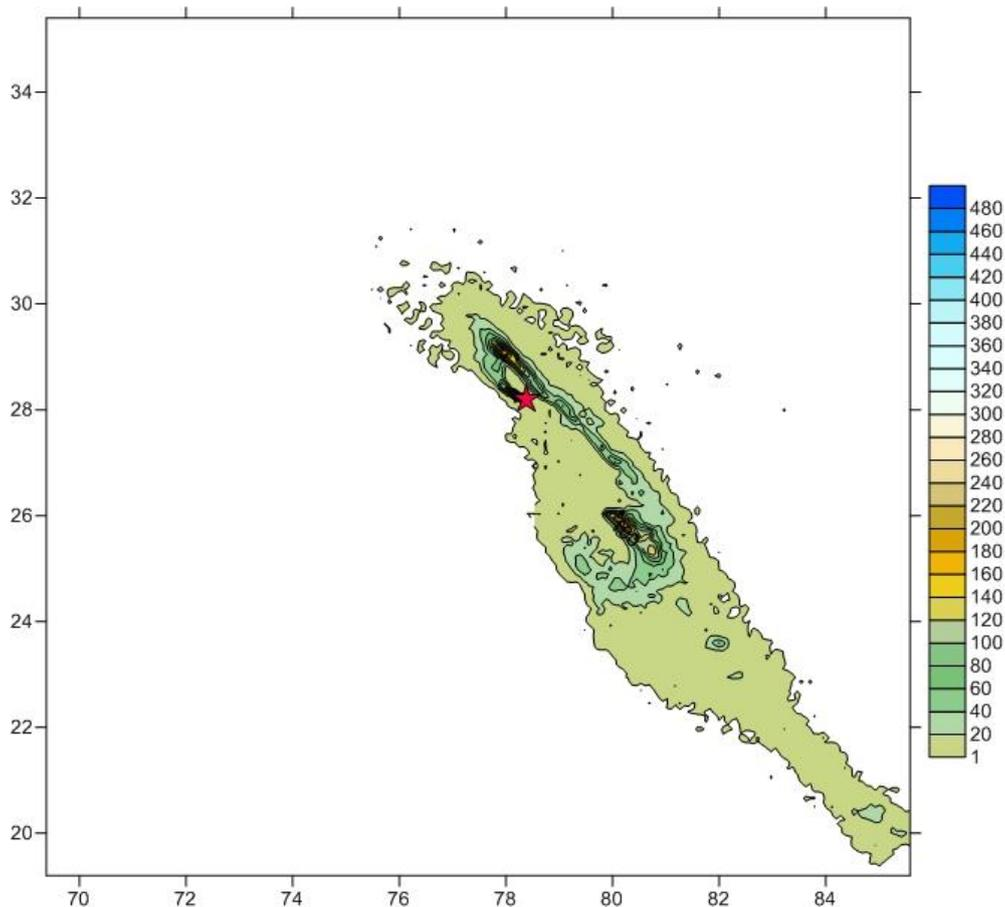
**Figure-3: Deposition pattern under completely non-homogeneous non-stationary meteorological condition for hypothetical release scenario using 4-dimensional meteorological data generated using NWP models**
