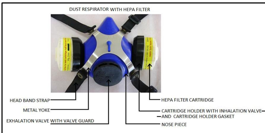
**Half Face Mask Dust Respirators:** This is an air-purifying respirator having half-face mask to cover nose and mouth. The newly modified face piece of the mask made up of silicon elastomer has soft internally rolled periphery, which assures comfortable and airtight fit on persons of widely varying facial contours and sizes. These Respirators are
