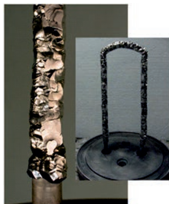
Fig. 3b: Zirconium crystal bar grown by iodide refining technique at BARC campus and the inset shows the crystal bar zirconium formed on U-shaped zirconium filament
