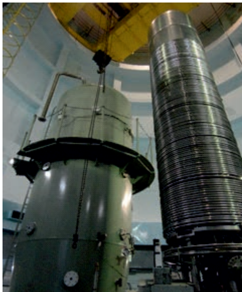
Fig. 3 (ii): Accelerating column of FOTIA at Van de Graaff, Trombay
