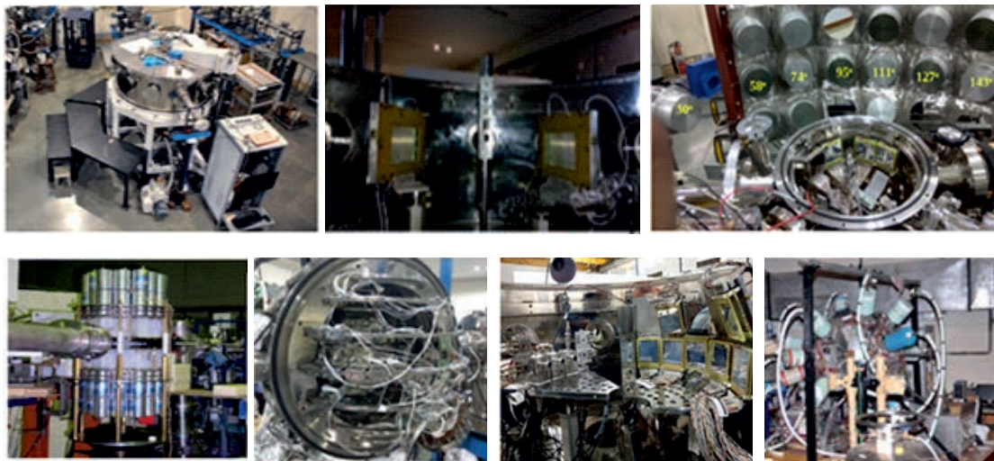
Fig. 6: Experimental facilities set up at PLF a) 1.5m diameter Multipurpose scattering chamber for reaction studies b) High granularity large solid angle strip detector array for charge particle detection c) Liquid scintillator array for neutron measurements d) \text{BaF}_2 array for high energy gamma rays measurements e) CsI array for light charge particle detection f) MWPC detectors for fission measurements g) High efficiency, high resolution Indian National Gamma Array (IGNA) for gamma ray measurements
