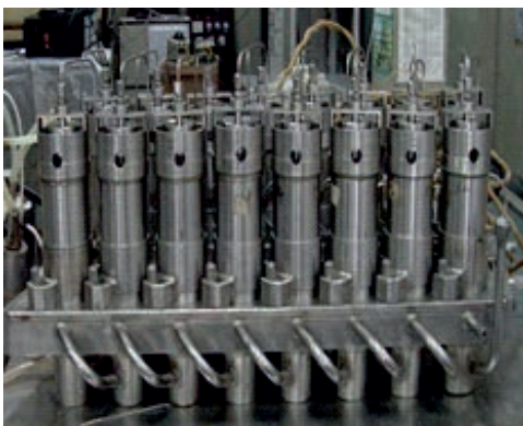
Centrifugal contactors used in CORAL plant
