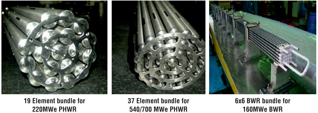
Fig.3: Three types of fuel sub-assemblies (bundles) fabricated in NFC
