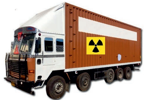
Fig. 3(b): Nuclear fuel is transported in trucks. 4 to 5 truck trips meet the annual nuclear fuel requirements of a typical 540 MWe Unit
