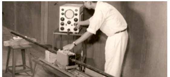
Fig. 7(b): Left Picture -Ultrasonic Testing (UT) of uranium billet for CIRUS Fuel. Right Picture-Eddy Current testing (ECT) of CIRUS rod. These techniques were developed at a time when there was no know how of this subject, in Indian industry. Later experts from BARC took active initiative in disseminating knowledge gained in this field, to specialists of other industries.
