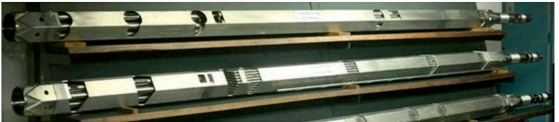
Fig. 12: Fuel assemblies for PFBR. It comprises of several pins each having uranium-plutonium MOX pellets. Since MOX is stable form of uranium and plutonium hence the fuel fabrication is carried directly in air media. However, leak tightness requirements are same as those of carbide fuel for FBTR (see Fig. 11) since radiological safety requirements are same for both. The fabrication is carried out at AFFF, BARC, Tarapur.
