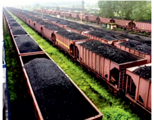
Fig. 2(b): Transportation of coal from mines to power station site is expensive and puts heavy demand on transportation infrastructure. A typical 500 MWe unit demands two 50 wagons goods train carrying 5000 tonnes of coal daily from mines to power station site. In the year 2021 about 700 million tonnes of coal was transported for different utility and captive power stations in India
