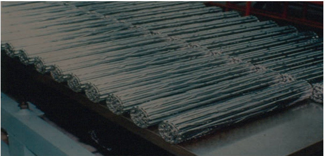
Fig. 8: First batch of Power Reactor Fuel for RAPS-1 PHWR was made in BARC and delivered during the period 1970 to 1971. Powder Metallurgy (PM) based technologies were established to fabricate fuel using natural uranium-dioxide. RAPS-1 achieved criticality in the year 1973. PHWR fuels are now fabricated at Nuclear Fuel Complex (NFC)-Hyderabad
