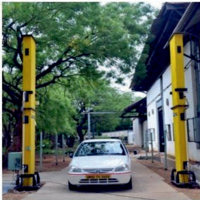
Fig.11: System developed for radiation monitoring of Vehicles and Cargos -VMS (ECIL has made many such VMS and installed them in the entrance and exit points of many facilities)
