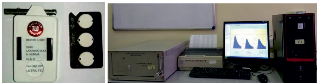
Fig.12: (a) TLD Badge and TLD Card (b) TLD Badge Reader along with PC and other Accessories
