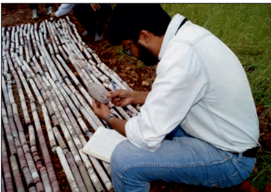
Fig. 6: On-site drill core examination by AMD geologist
