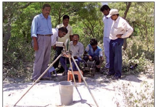
Fig. 7: Gamma ray logging of borehole
