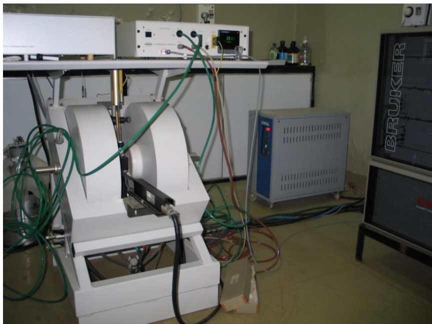
Fig. 1: EPR spectrometer facility at FIPLY
