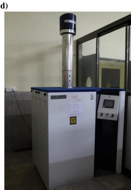
Fig. 5: (a) Gamma Chamber (Gamma Cell 220) of FTD, BARC commissioned in 1967 in collaboration with AECL, Canada, (b) Gamma Cell 900 designed by BRIT, DAE commissioned in 1995, (c) Gamma Chamber 5000 of BRIT, DAE commissioned in 2005, (d) Gamma Chamber 5000 designed by BRIT, DAE commissioned in 2017.
