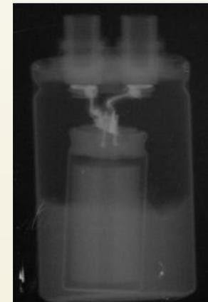
Flash X-ray systems provide a unique method of imaging very fast events which cannot be captured using normal photographic techniques. X-ray images can be obtained in few tens of nanoseconds even through smoke, fire and metal. Harder than those produced for Medical purposes and suitable for dynamic radiography. Have higher penetration power and can penetrate thick steel containers.
