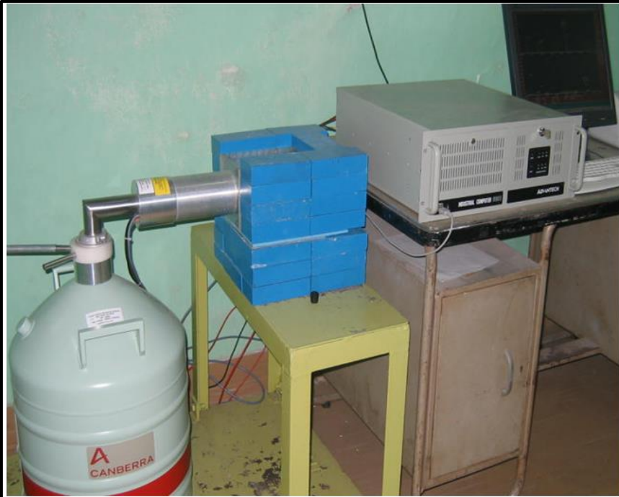
HPGe Detector set-up for foil activity measurement
