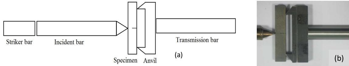
Figure 1. (a) Schematic of modified SHPB arrangement, (b) Specimen loaded in SHPB
