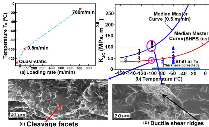
Figure 2. (a) Variation of reference temperature  $T_0$  with loading rate, (b) comparison of master curve at 0.5m/min and 700m/min and shift in  $T_0$  (c) Cleavage fracture at -100 °C at 700m/min and (d) ductile ridges at 0.5m/min at -100 °C
