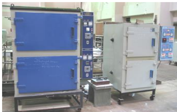
Figure 1: Thermal Ageing Facility
