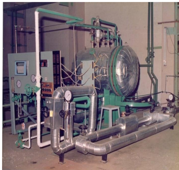
Figure 2: LOCA chamber for equipment qualification
