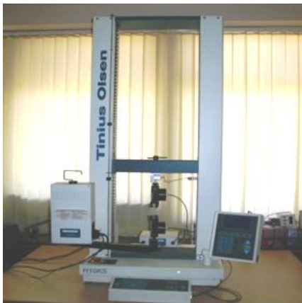
Figure 4: Tensile test facility
