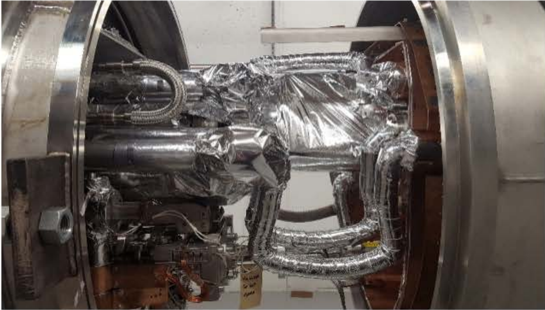
Feed Cap & End Cap Internal Cryogenic lines connection with Cryomodule
