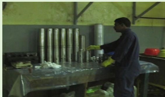
Decontaminated SS plugs
