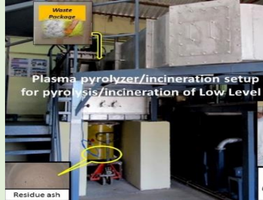
PLASMA PYROLYSIS/INCINERATION Volume Reduction Factor: > 30
