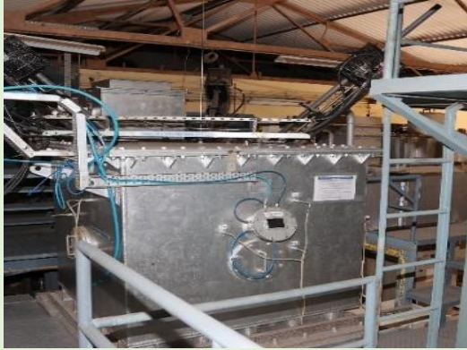
PLASMA PYROLYSIS/INCINERATION Volume Reduction Factor: > 30
