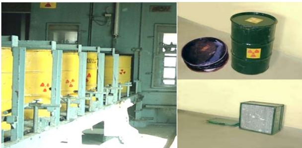
COMPACTION SYSTEM Volume Reduction Factor: 3 - 5
