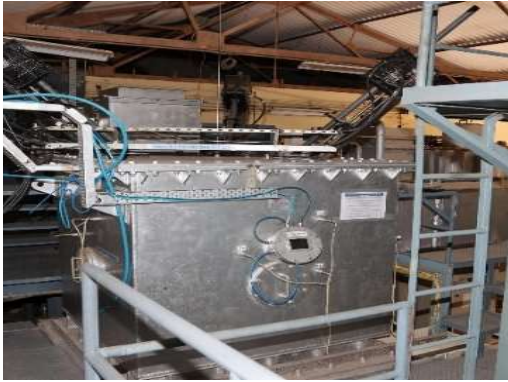
PLASMA PYROLYSIS/INCINERATION Volume Reduction Factor: > 30
