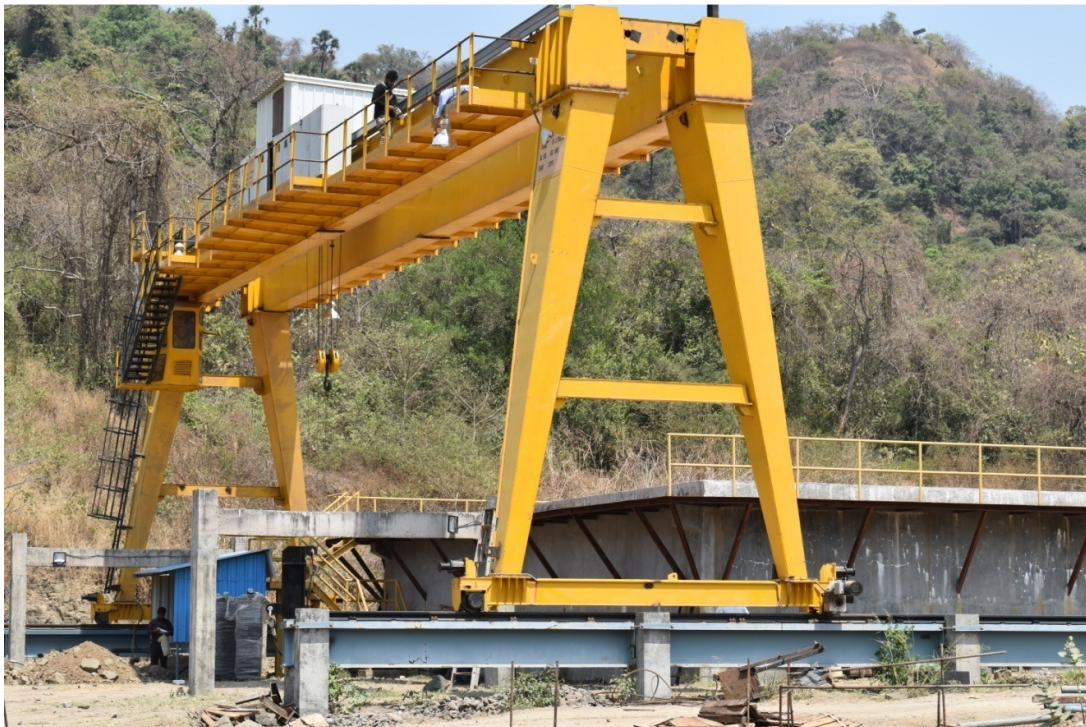
Fully Assembled 10/2 Tonne, 26 mtr.span outdoor duty Gantry Crane at RSMS
