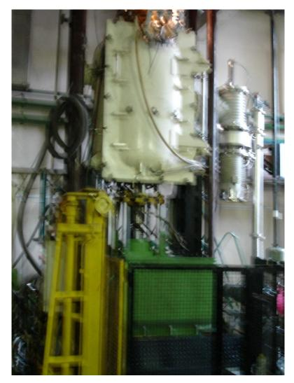
Capacity: 100 T Pressing condition: 2100 °C, 30 MPa, Vacuum: ~10<sup>-3</sup> mbar Induction heating
