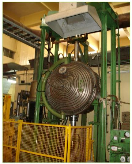
Capacity: 30 T Pressing condition: 1500 °C, 30 MPa, Vacuum: ~10<sup>-3</sup> mbar Induction heating
