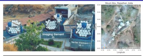
**Location** - Mt. Abu, Rajasthan, India **Light collector area**  $\sim 9.5~\text{m}^2$  **Pixel size** =  $0.318^0$  **Trigger FOV**  $\sim 3.40^0$  X  $3.40^0$  **Mount** - Alt-Azm **Back end electronics**-NIM/CAMAC
