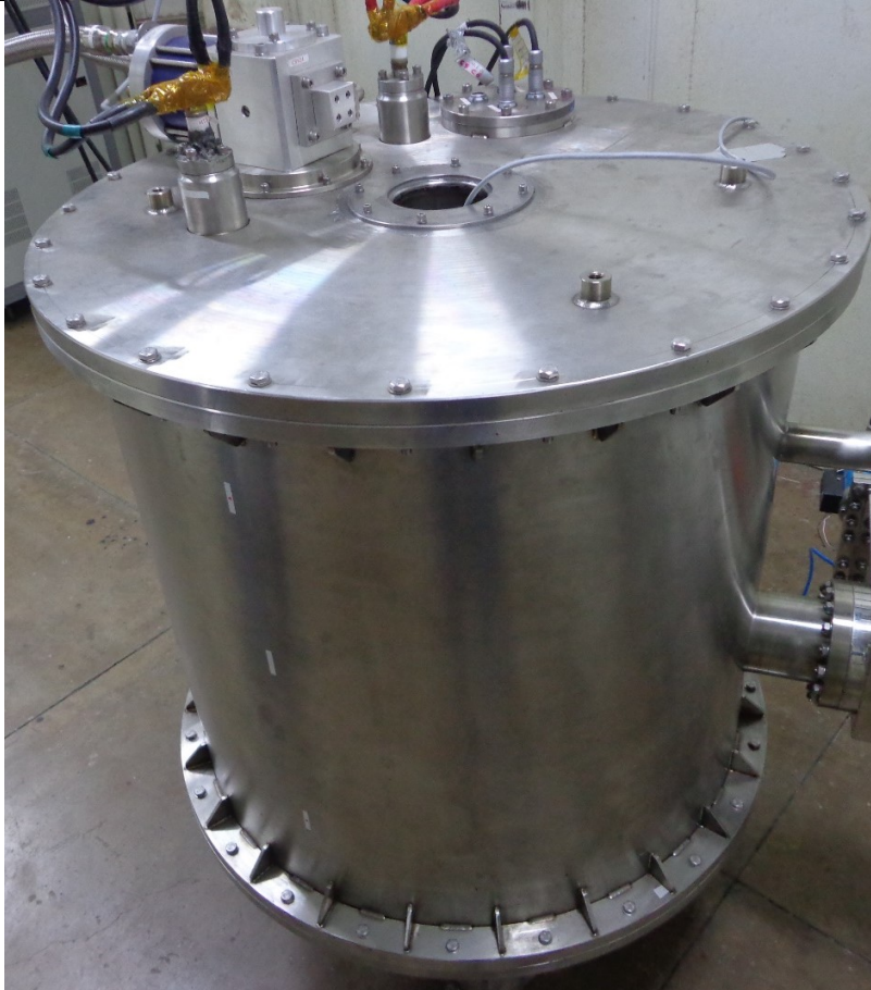
130mm diameter warm bore cryogen free magnet for HGMS
