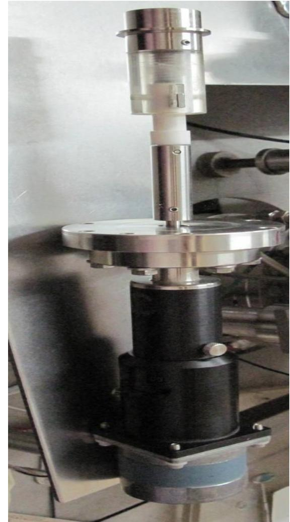
**Sample Probe attached to a Stepper Motor**
