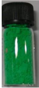
\text{UF}_4 produced from fine \text{UO}_3 powder
