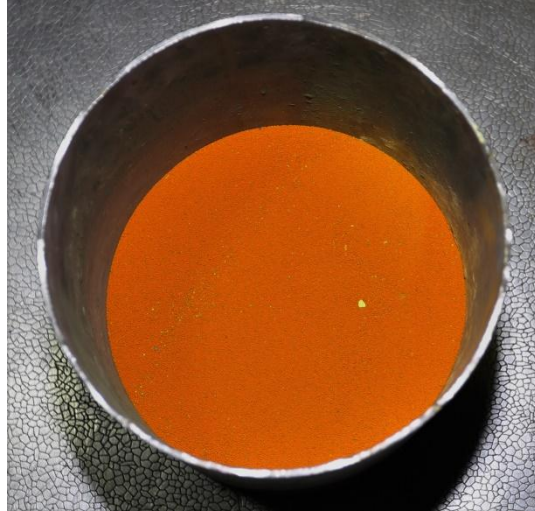
\text{UO}_3 produced in direct denitration process
