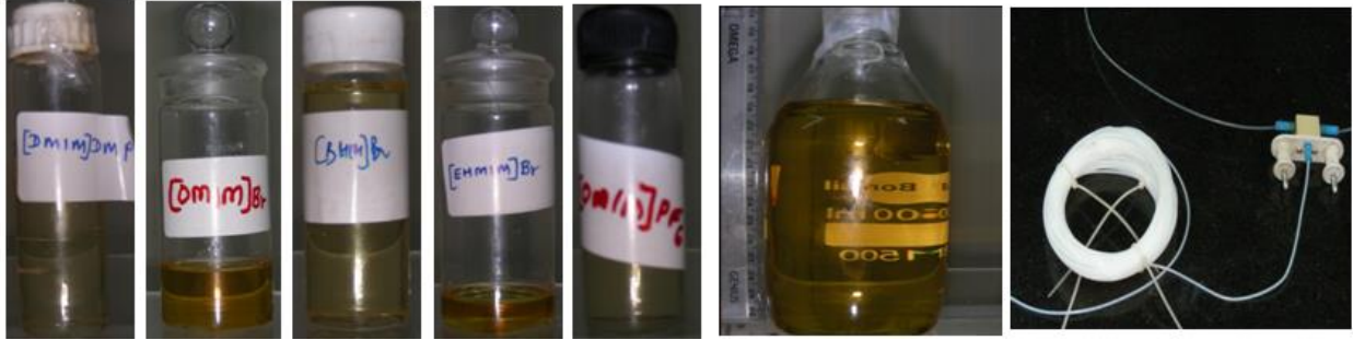
Different types of ionic liquids synthesized in microreactor
