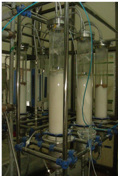
Glass column purification system for crown ether
