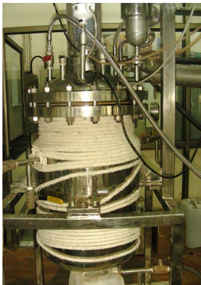
85 L Hastelloy reactor for crown ether precursor synthesis
