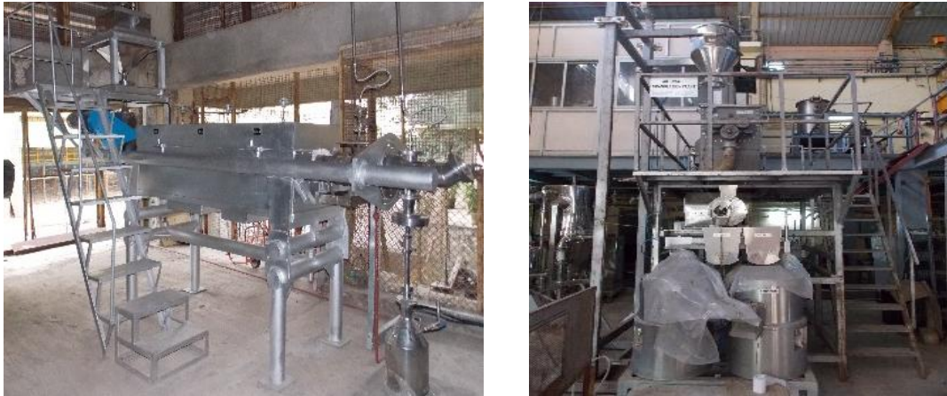
Fig. 1 (a) Rotary reactor (b) automated granulation system for the synthesis and fabrication of pebbles of solid breeder materials viz. \text{Li}_2\text{TiO}_3 and \text{Li}_4\text{SiO}_4
