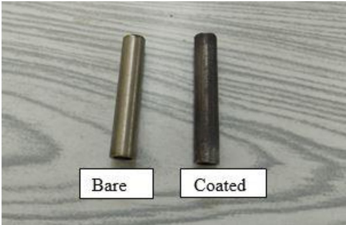
Alumina coating on SS 304 tubular substrate
