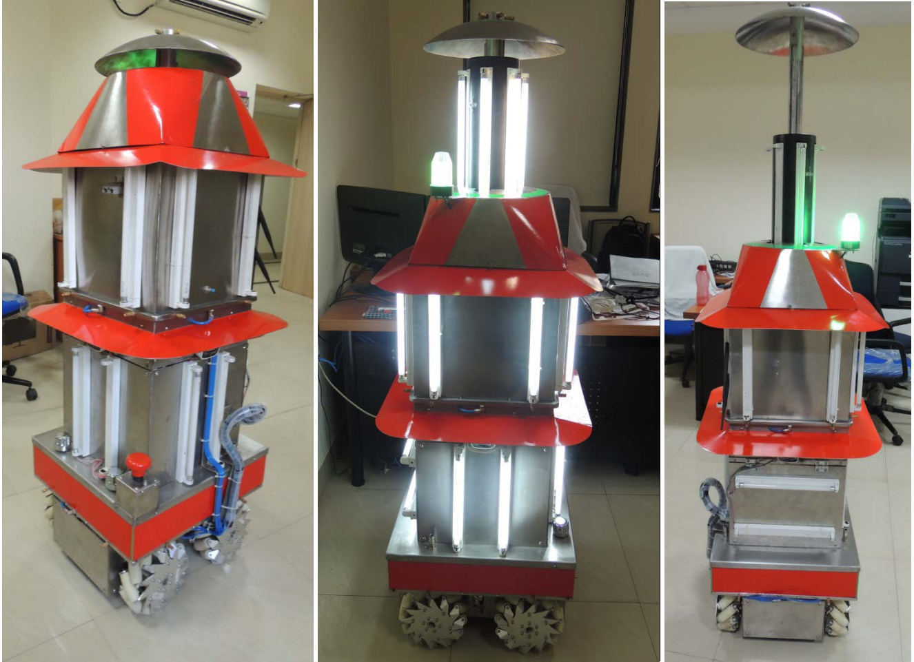
Figure: (left) Robot in retracted condition; (middle) UV-C based disinfection; (right) Spray based disinfection
