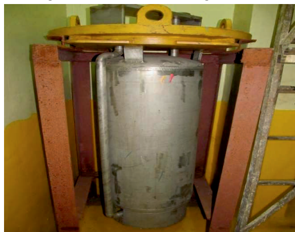
Ion Exchange column of 100 litre bed volume without shielding.
