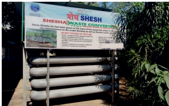
A portable Nisargruna Plant with 50kg daily capacity.
