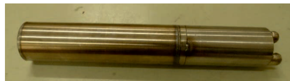
Natural boron coated parallel plate ionization chamber.
