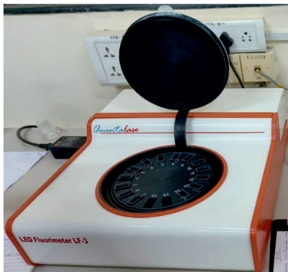
Multi cuvette LED fluorimetry system.
