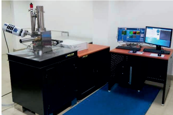
Tungsten filament-based SEM.
