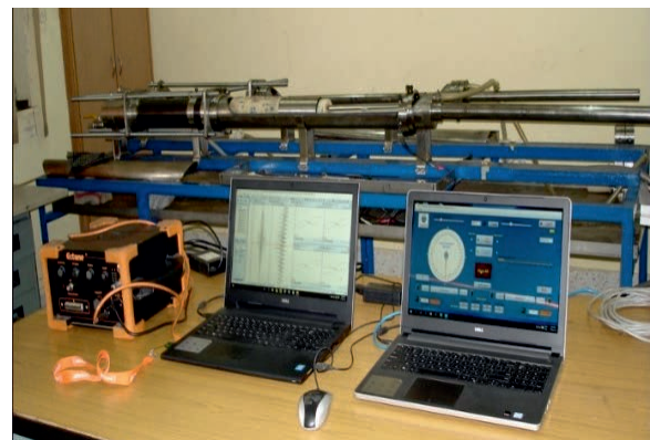
Set-up for Testing of Eddy Current based Inspection Tool in Horizontal Calibration Facility.
