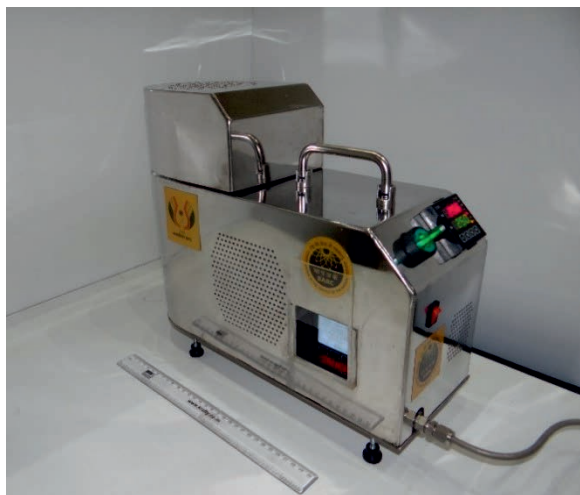
Prototype of portable hydrogen storage gas dispenser for laboratory applications.
