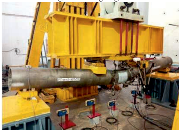
Fracture tests being carried out on full scale pipe weld with crack.
