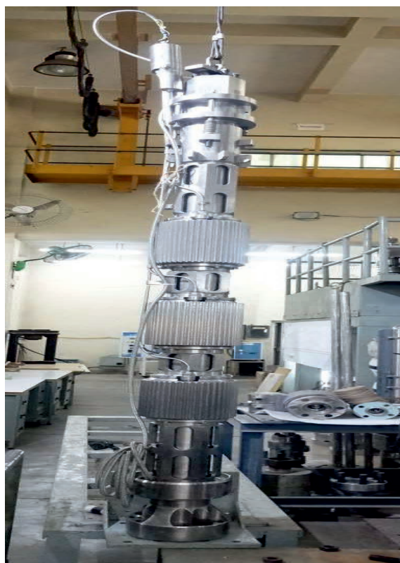
The Magnetic Jack type Reactivity Control Mechanism.
