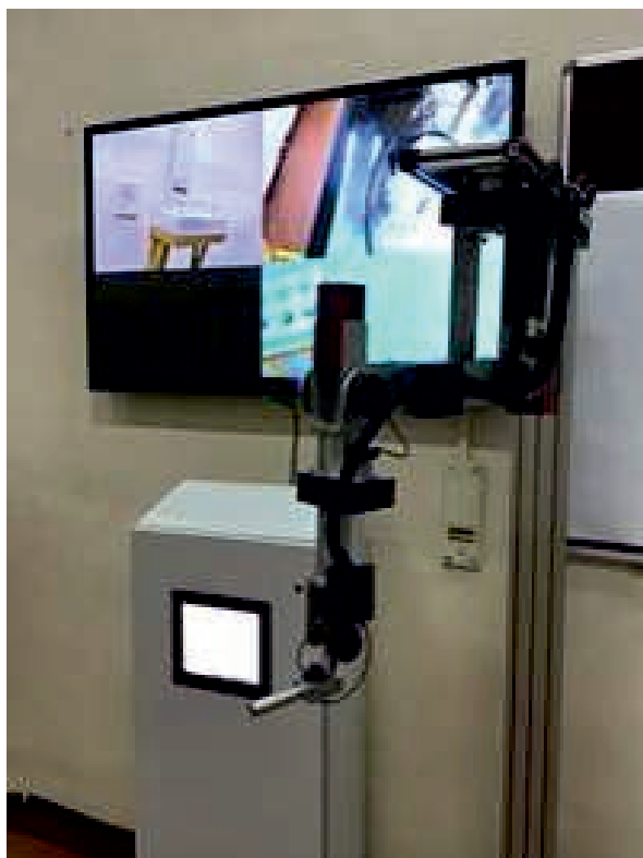
The Master arm at remote control console of Iodine-131 vial handling system.
