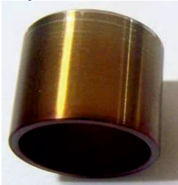
SiC thin film deposited on SS Tube via PECVD.
