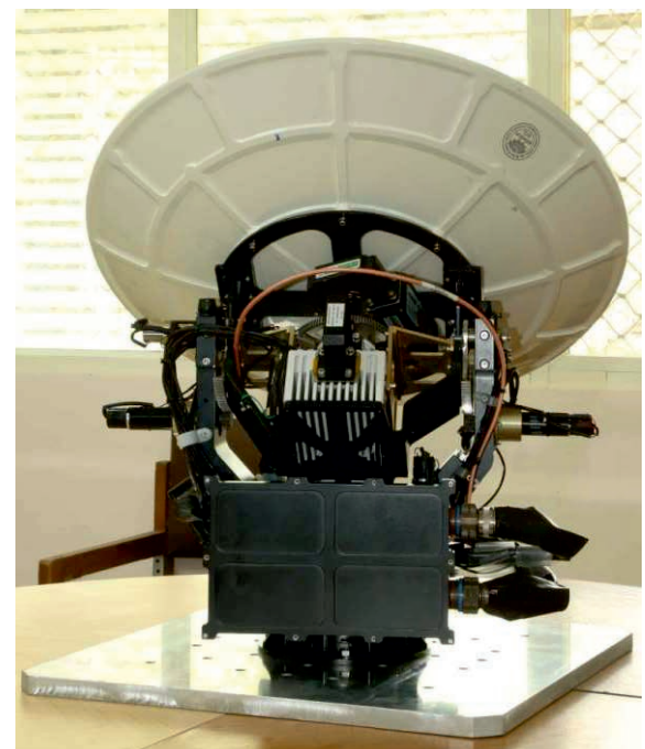
The 0.6M Airborne Satcom Terminal ET with ACU.
