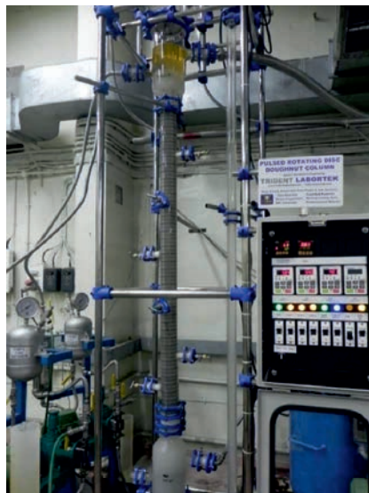
Extraction of Zr is in Pulsed Disc and Doughnut Column (PDDC) of 3-inch diameter.
