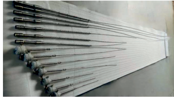
Heated Junction Thermocouple based discrete level sensors.
