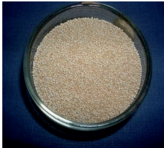
The adsorbent used for removal of carbon dioxide from air.
