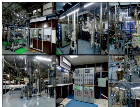
Integrated pilot scale Copper-Chlorine (Cu-Cl) thermochemical cycle facility with design capacity of 150 NL/h hydrogen.
