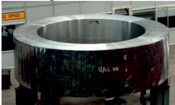
APURVA Steel Forging: 750 mm thick Ring Forging for Flange Area of RPV-OD5300 x ID3800 x 700L.
