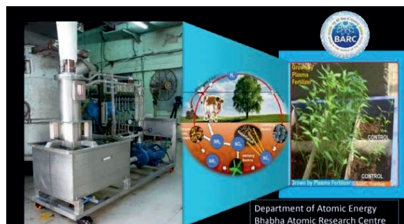
A portable air plasma system for fast synthesis of aqueous Nitrate & Nitrite fertilizers.
