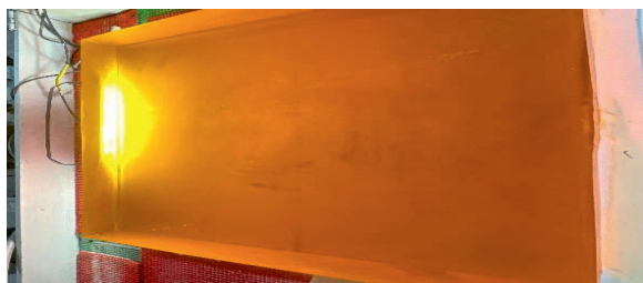
Casted glass slab of 740mm x 740 mm x 200 mm thk (5.2 g/cc density).
