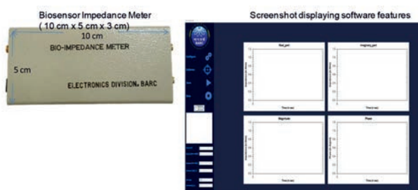
Hand-held biosensor for the detection of cancerous cells.
