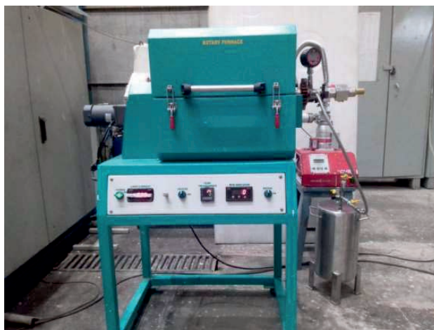
0.5 kg scale \text{MgH}_2 synthesis set-up developed in-house.
