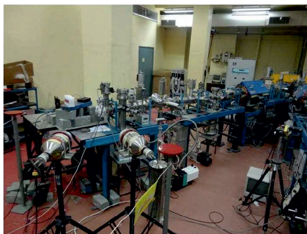
Experimental set-up for fast neutron induced fission experiments at FOTIA.
