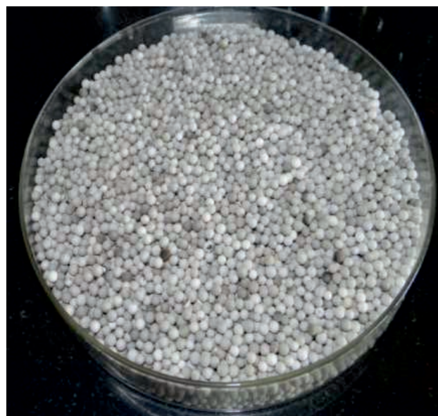
1% Pd on Alumina catalyst for ultra-purification of AWE products.
