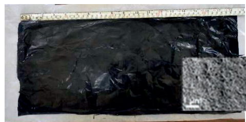
Self-assembled CNT sheet (inset SEM image).
