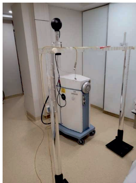
Experimental set-up used for characterisation of this ionization chamber.
