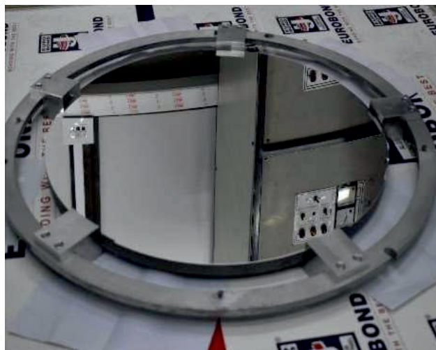
High reflection thin film coated 60 cm dia. TACTIC telescope mirror.
