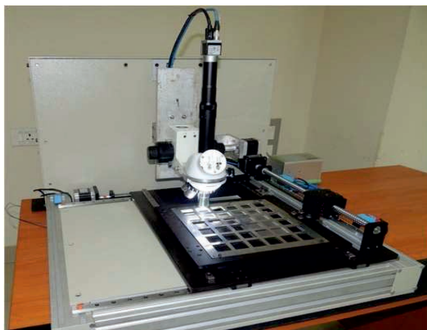
Microscope based Image Analyzer System.
