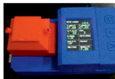
CNT based VOC sensing device.
