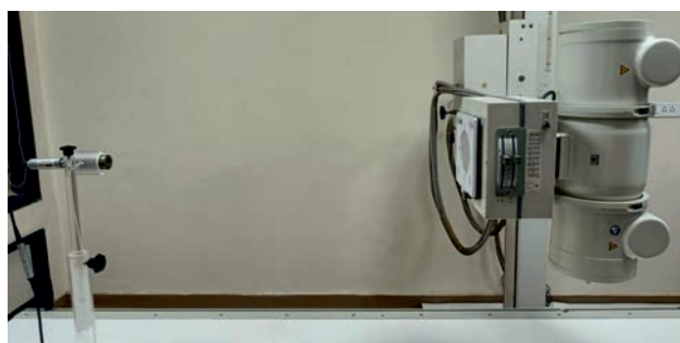
Experimental set-up used for measurement of diagnostic x-ray beam spectrum.
