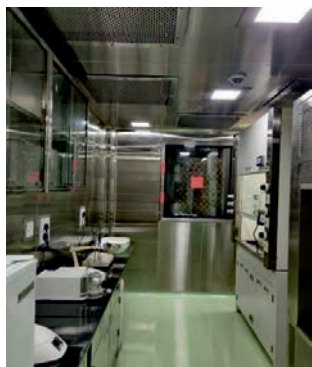
A Clean room (ISO 7) with clean bench facility (ISO 5) was established in BARC.
