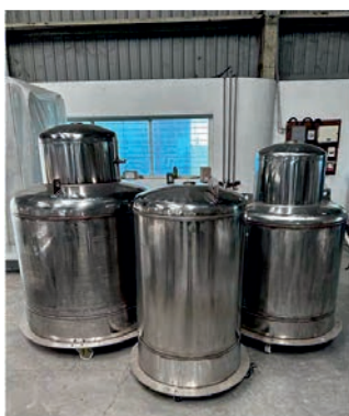
Final Helium Dewars after fabrication.
