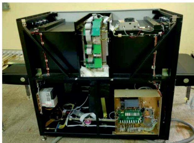
XBIS Electronics mounted on X-ray machine.
