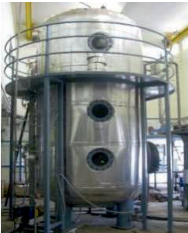
WASIF-II Test Vessel for Suppression Pool Simulation studies.
