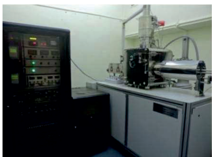
10kW Electron Beam Melting machine installed in BARC.
