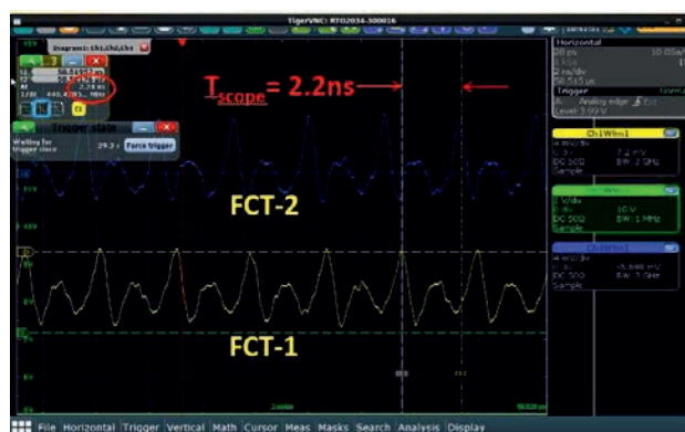
The time difference between the two FCT signals measured to be 2.2 ns.
