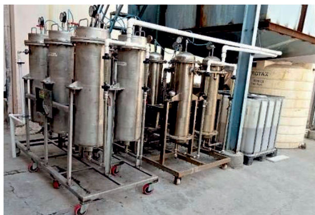
The 75 KLD capacity demonstration plant for de-coloration of dye industry wastewater.
