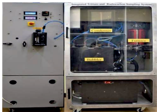
Prototype Integrated Tritium and Radiocarbon Sampling System developed in BARC.
