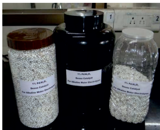
8kg batch of supported noble metal catalyst.
