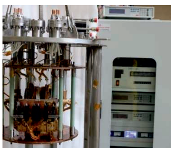
Test stand for cryogenic testing of superconducting magnet assembly.
