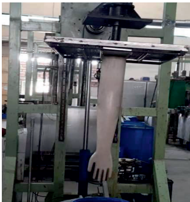
Set-up created in BARC for development of Gauntlets for radioactive applications.
