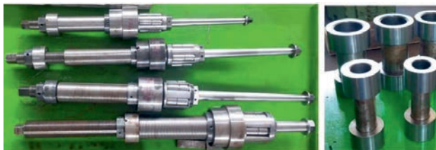
Rolling Tools & Rolled Joint Specimen.
