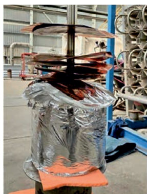
Helium Dewar showing thermal shield and MLI.
