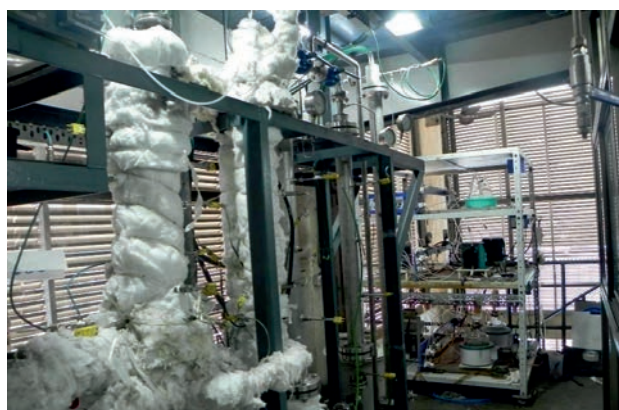
A first-of-its kind integrated metallic bench scale Copper-Chlorine facility in BARC.
