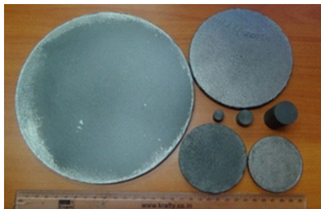
Illustration of the \text{TiB}_2 powder and dense component made from it at BARC
