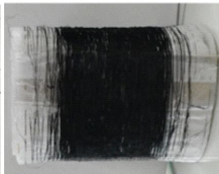
Fig.3: Continuously spun CNT fibre.
