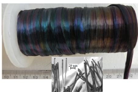
Fig.4: SiC coated Carbon fibre. Inset shows the micrograph of the fibre.
