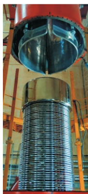
Electron Beam accelerator for wastewater treatment (Right).
