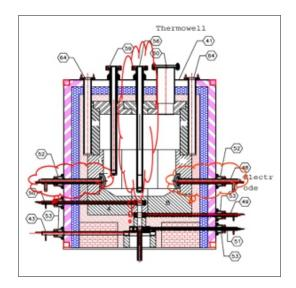
The schematic of Joule Heated Ceramic Melter (JHCM). The operational life of JHCM is primarily limited by degradation of heating elements and internal components, exposed to harsh conditions of high radiation, continuous corrosive attack, and sustained temperatures upwards of 950°C.
