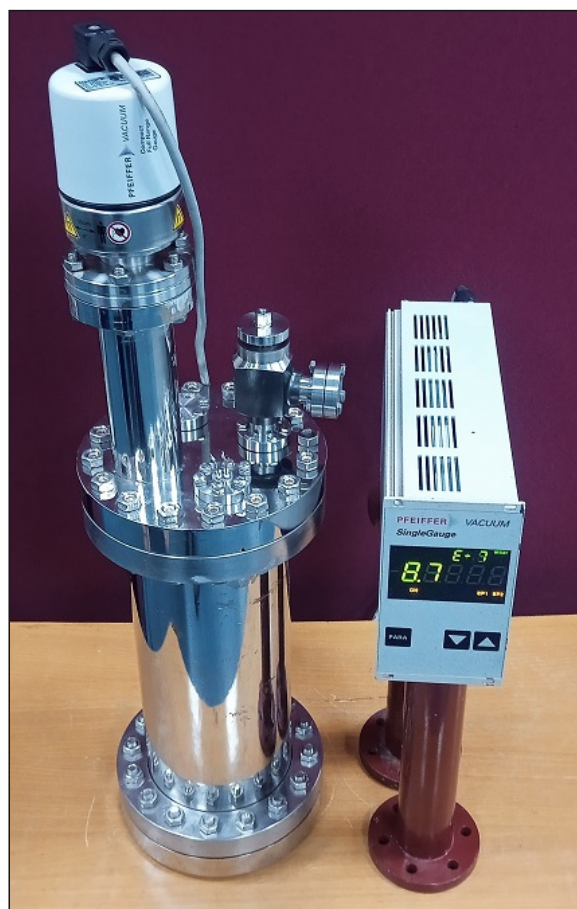
Fig.6: Photograph of the sealed off vacuum chamber.
