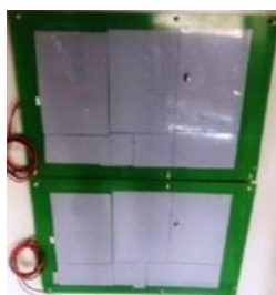
Fig.4: Heater PCBs with heat pads.
