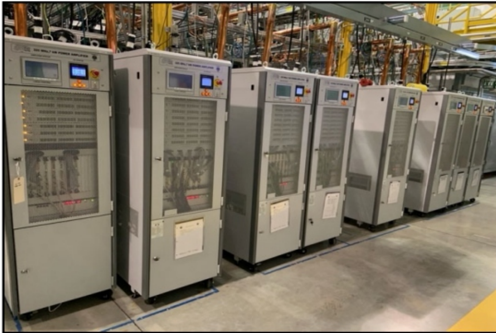
Fig.3: EIGHT SSAs coupled to SSR1 of PIP2IT @Fermilab (Photo Courtesy of Fermilab, USA).
