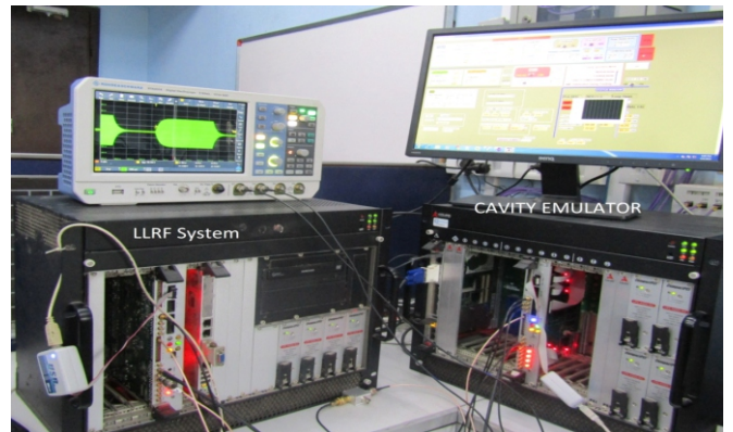
Fig.5: LLRF integration with Emulator.
