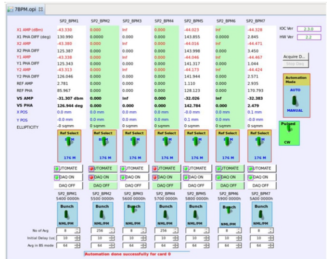
Fig.5: Command control application screen for control of 7 BPM systems.
