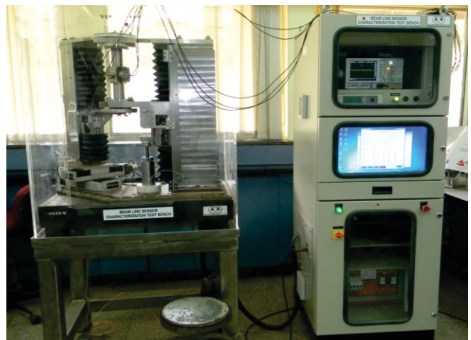
Fig.6: BPM characterization test bench at ACnD, BARC.
