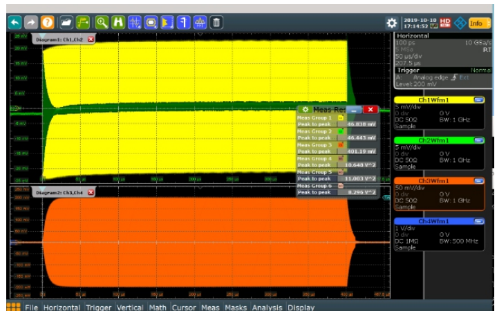
Fig.9: RF Power Waveform of SSA and RF waveforms recorded after RF amplifier was integrated with buncher.
