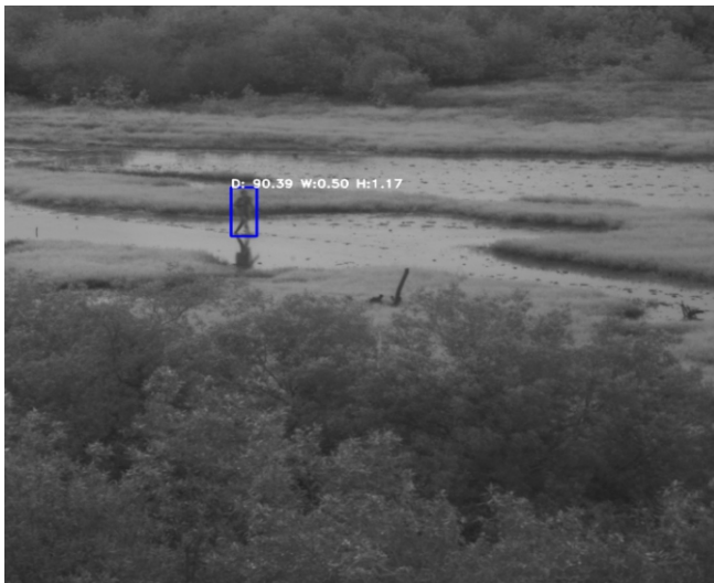
Fig.2: Image showing a blue coloured bounding box marked over a detected intrusion. The depth, width and height (in meters) of the intrusion are also indicated over the bounding box as text.
