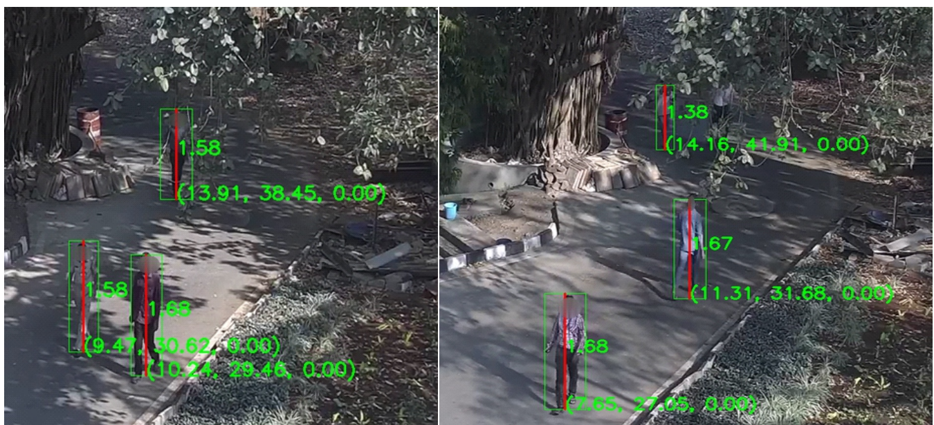
Fig.3: Images showing intrusion with their 3D coordinates of feet and height(in meters) of the intrusion.
