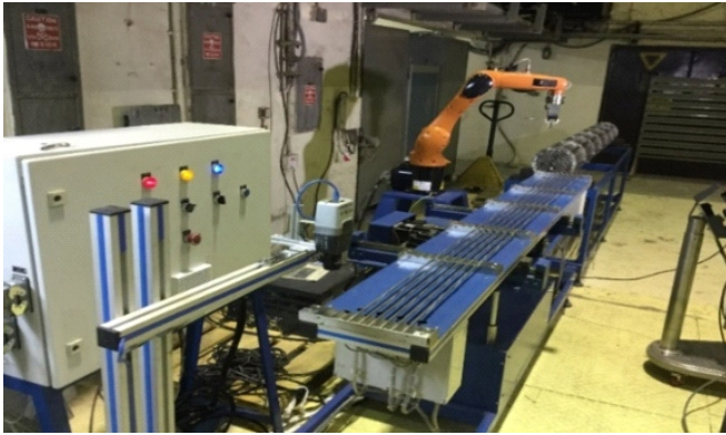
Fig.10: Robotic system installed at PFBR fabrication facility.
