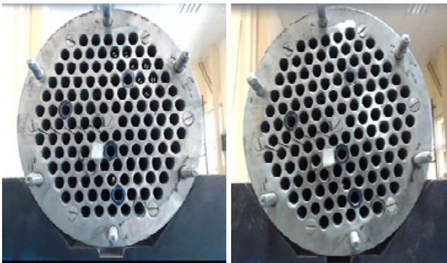
Fig.8: Orientation error because of variable transport magazine placement.
