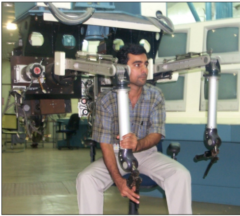
Fig.6: Control station and master arm of indigenous Servo Manipulator at WIP, Trombay.
