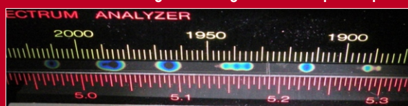
CO laser emission spectra in 5 \mu\text{m} region from the gas discharge for 90% output couplers
